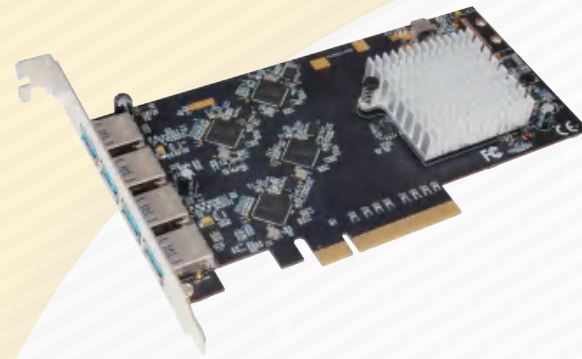
U-2500 PCIe Quad Bus USB 10Gbps Host Adapter (4x USB-A 10Gbps Ports)
