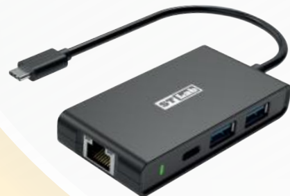
U-2670 USB-C 10Gbps Multiport Adapter (2.5GbE + 1X USB-C 10Gbps + 2x USB-A 10Gbps)
