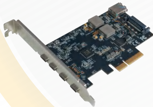
U-2330 PCIe 5 Ports USB10Gbps Host Adapter (4x USB-C 10Gbps + 1x USB-A Internal Ports)
